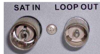
Typical Antenna Loop
